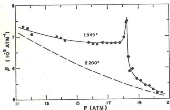
FIG. 4. Compressibility of liquid He<sup>4</sup> at 1.95 and 2.200°K.
