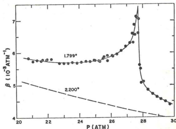
FIG. 5. Compressibility of liquid He<sup>4</sup> at 1.80 and 2.200°K.
