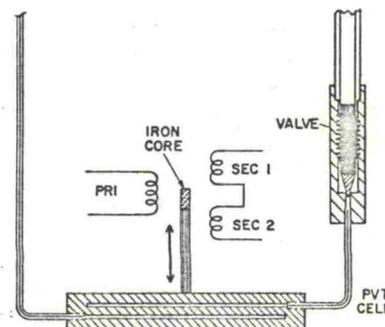
FIG. 1. The  $P$ - $V$ - $T$  cell.
