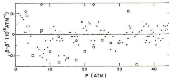
FIG. 3. Deviations of liquid  $\text{He}^4$  compressibility at  $2.200^\circ\text{K}$  from  $0.30 \times 10^{-3} + (72.0 \times 6.66P)^{-1}$ . ● present measurements; ○ derived from density data of Keesom and Keesom (Ref. 1); □ derived from density of Edeskuty and Sherman (Ref. 5).
